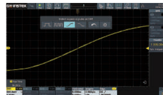
Detecting Square or Pulse Waves, the Second-level Menu Optimizes Pulse Width and Edge Timing Measurements
